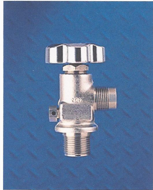
6074 SERIES - 303 SS PACKLESS DIAPHRAGM VALVES
