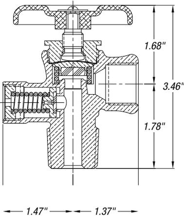
**Sherwood's 1032 Series is designed for use in liquefied gas applications, including refrigerants and flammables, and is especially suitable for propane, butane and fuel-gas applications but also sterilant gas applications.**
