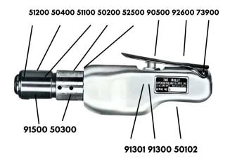
Before using a new tool, pour a small amount of oil into the air inlet, connect the hose, and run the tool momentarily to distribute the oil into all of the working parts. The best oil to use is Superior Pneumatic Oil, but if Superior Pneumatic Oil is not available, do not use oil heavier than SAE #10. Thereafter, insert several drops of oil into the air inlet after every two or three hours of operation. If the unit is in constant use, it must be equipped with an airline lubricator and filter.
