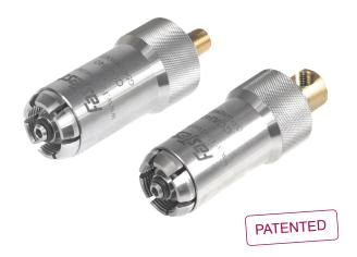
FasTest's G540 medical oxygen and industrial connector is simple to use with a no twist, no turn approach to filling. Simply connect onto your CGA 540 valve and lock into place with a forward movement of the sleeve and you are ready to fill the medical or industrial oxygen cylinder in a matter of seconds.
